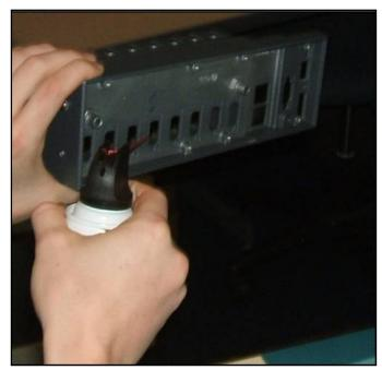
Removing debris from the chassis with compressed air
