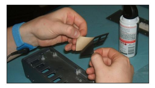
3. Lightly place the gasket in the chassis adhesive side down making sure it is aligned correctly according to the following diagram.
