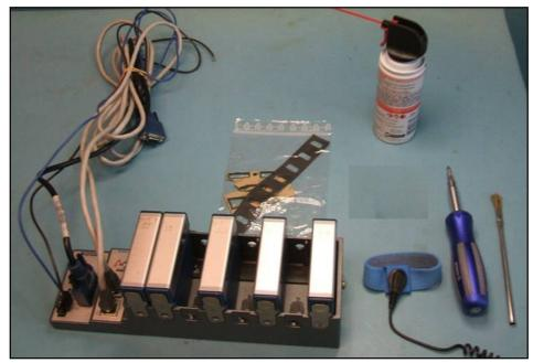
cRIO-FRC, Gasket Kit, ESD wristband, compressed air, #1 screwdriver, and clean paintbrush
