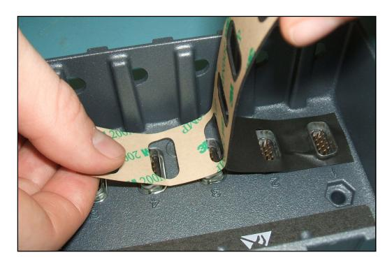
5. When the gasket is in place around all connectors, go back over it and firmly press it into place with a soft, blunt tool.
